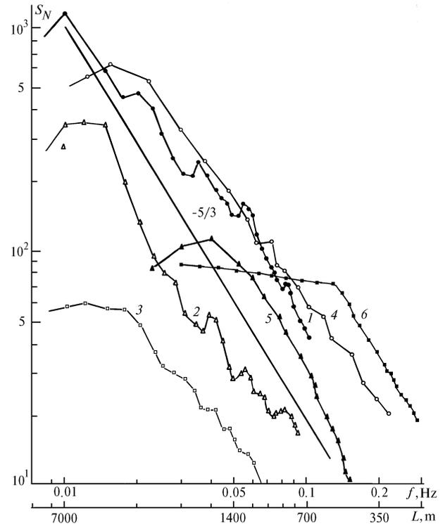
FIG. 8. Spectral density of the aerosol number density fluctuations ( $d \geq 0.4 \mu\text{m}$ ) at altitudes of 500 (1), 2000 (2), and 4500 m (3) and at altitude of 2500 m for particles of  $d \geq 0.4$  (4), 1.0 (5), and 4.0  $\mu\text{m}$  (6).
