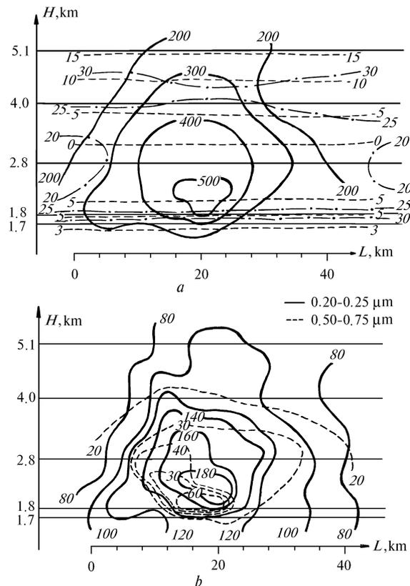
FIG. 10. Noncondensational aerosol cloud: a) distribution of temperature (---), humidity (- · -), and aerosol particles number density (bold solid line); aircraft flight levels (solid line); b) particle density distribution:  $r = 0.20\text{--}0.25 \mu\text{m}$  (—) and  $r = 0.50\text{--}0.75 \mu\text{m}$  (---).
