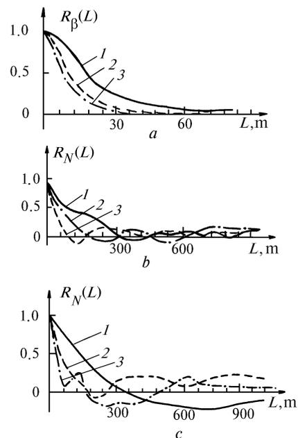
FIG. 6. Spatial normalized autocorrelation functions of: a) backscattering coefficient ( $\lambda = 0.7 \mu\text{m}$ ) at altitudes of 400 (1), 1500 (2), and 3200 m (3); b) number density ( $d \geq 0.4 \mu\text{m}$ ) at altitudes of 500 (1), 2600 (2), and 4600 m (3); and, c) at altitude of 1500 m for particles of  $d \geq 0.4$  (1), 0.7 (2), and 1  $\mu\text{m}$  (3).
