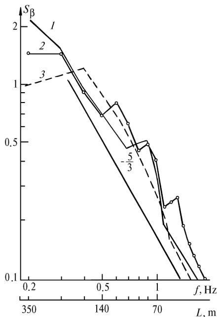
FIG. 7. Spectral density of backscattering coefficient fluctuations ( $\lambda = 0.7 \mu\text{m}$ ) at altitudes of 500 (1), 3000 (2), and 4600 m (3).
