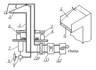
FIG. 1. Design of the sampler. The scheme of the nozzle is shown in the upper right corner. 1) variable area; 2) movable damper.
