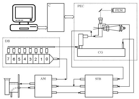
Fig. 4. Schematic diagram of the airborne ADB: DB is module of the diffusion battery, PEC is photoelectric counter, CG is condensation grower, STB is stabilizer of airflow rate, AM is aspiration module, C is controller.
