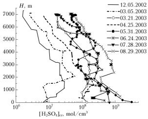
**Fig. 9.** Model profiles of the critical concentration of sulfur acid calculated by Eq. (5) using the data of airborne sounding over the south of Western Siberia.
