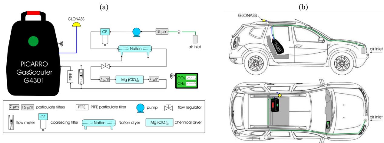
Figure 1. Schematic diagram of the drying unit (a) and the G4301 installation in a vehicle (b).
