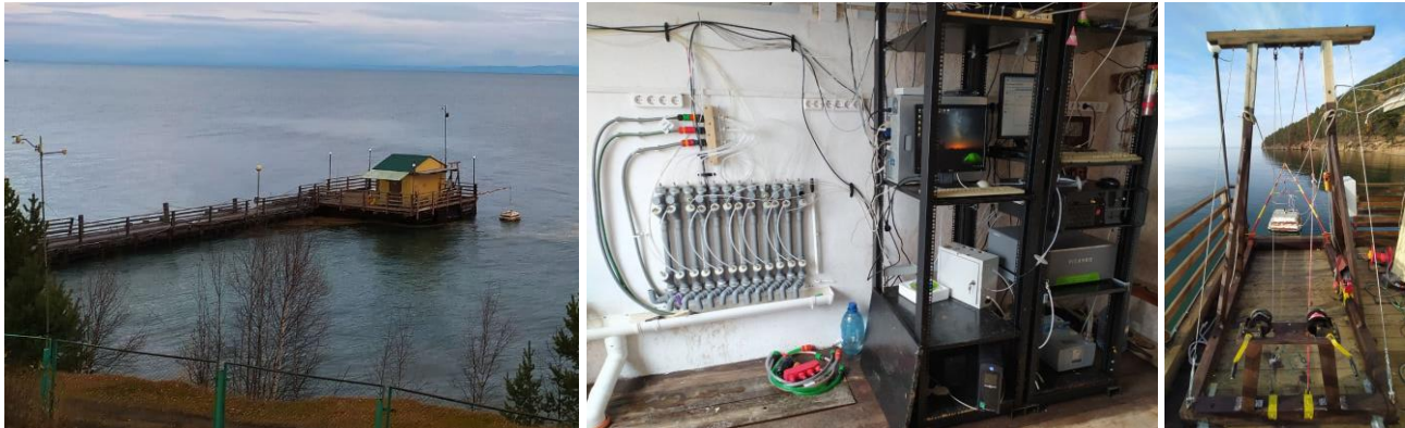
Fig. 1. Baikal Atmospheric-Limnological Observatory (BALO) on the pier; BALO interior: equilibrator and gas-analysis equipment; Semi-submersible chamber in the accumulation mode.
