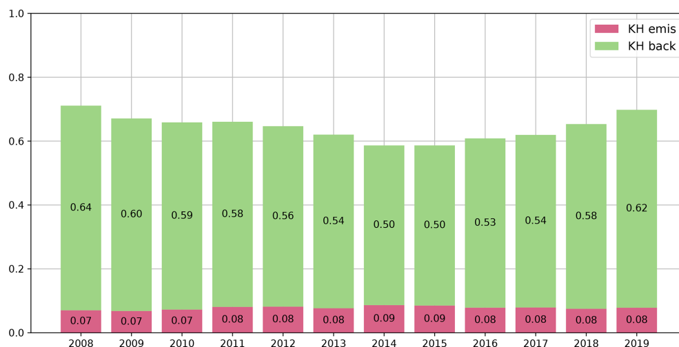
Figure 8. Traces of influence matrices divided by the number of available measurements of the corresponding year. See Sect. 2.1 for details on the computation of the influence matrix. The closer \text{tr}(\mathbf{KH}) is to 1, the more observations are used in the inversion.
